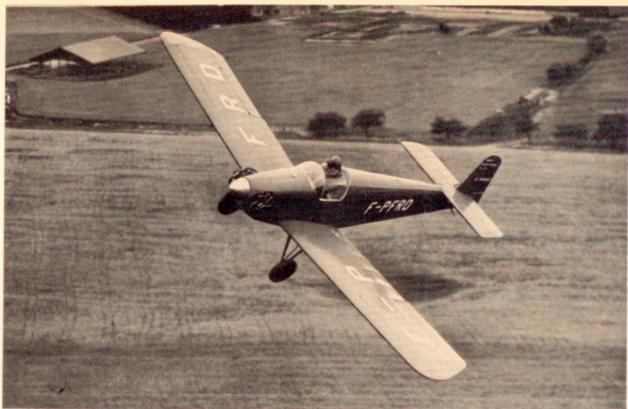
France leads the European market for home-built sportscraft. The Draine Turbulent, above, has a 40 h.p. adapted Volkswagen power plant. Also built commercially in France, Britain, Germany and Spain, it sells for about $3,000
