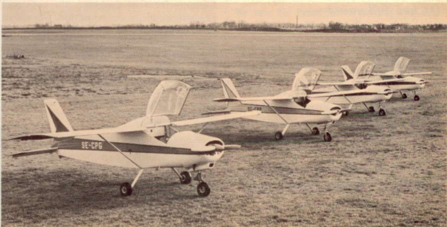
Popular low-cost sport plane is the craft above, manufactured in both Germany (Bolkow Junior) and Sweden (Malmo Junior). It cruises at more than 115 m.p.h., has a 65 h.p. engine
